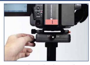
Using the Side-to-Side Adjuster Knob, align your Side-to-Side mark with the CENTER of the Post.
