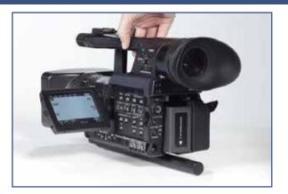
Rotate the camera 90° and find the **Side-to-Side** balance point. When found, mark the point on the camera using a piece of tape.
